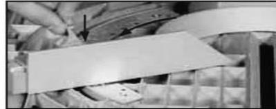
Ensure the saw head bevel tilt is  $0^{\circ}$  to the saw table. (1)
